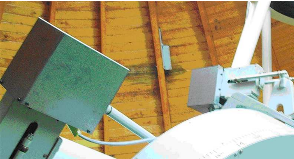
Fig. 1. The test set mounted directly on the worm-gear boxes of the telescope
