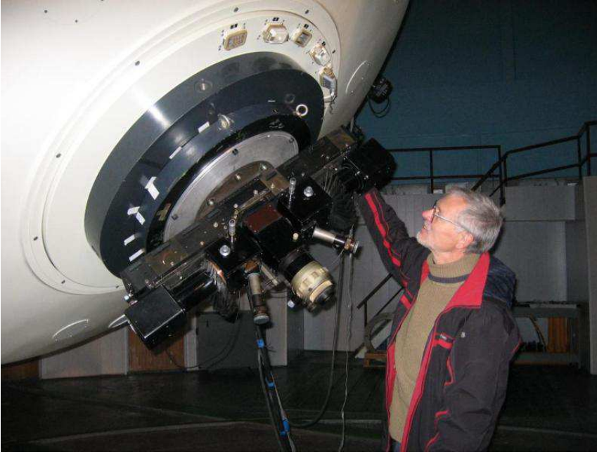
Fig. 15. The high-speed two channel UBVRI photometer with photo-multipliers
