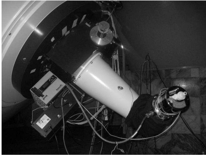
**Fig. 8.** The focal reducer of the 2-m telescope with TV guiding system
