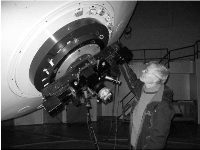
**Fig. 7.** The high speed two-channel UVBRI photometer with photo-multipliers
