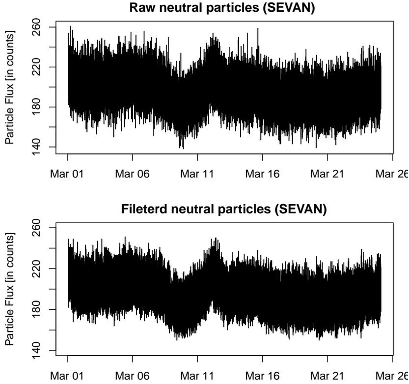
**Fig. 3.** Graphics of raw and filtered data for neutral particles measured with SEVAN for the period March 1- March 25 2012. The first hour of March 1 is missing from filtered data due to filter calibration.
