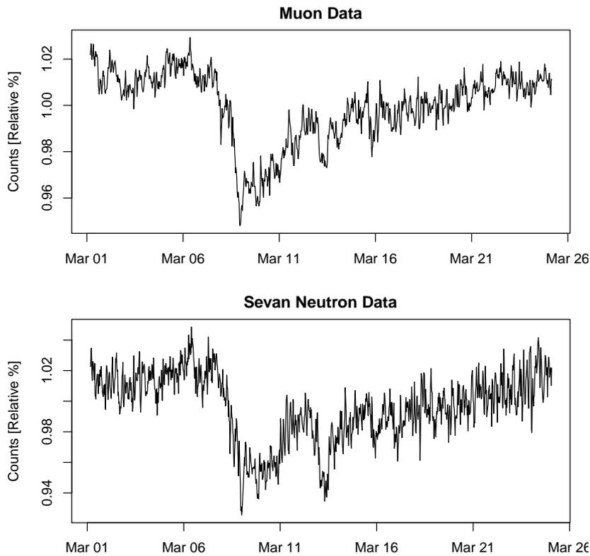
**Fig. 4.** 30 minute averages for neutrons and muons measured at Moussala. The neutrons are measured by SEVAN equipment for period March 1 0000UTC until March 25 2359UTC. The data from muon telescope is for period 0000UTC until March 30 2359UTC
