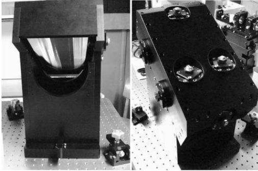
**Fig. 4.** A view of a typical echelle grating in a holder (BESO, Steiner [2006]). The small inclination of the working surface to the incident light is a characteristic feature for these gratings.
