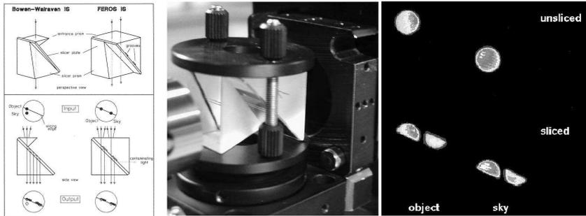
**Fig. 5.** Bowen-Walraven image slicer principle (left) and a sample performance (BESO, Steiner [2006])
